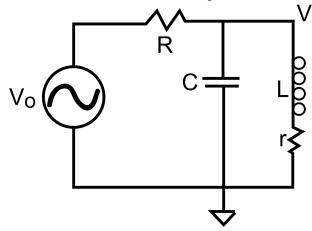
The equivalent impedance of the (L+r)||C| circuit is
