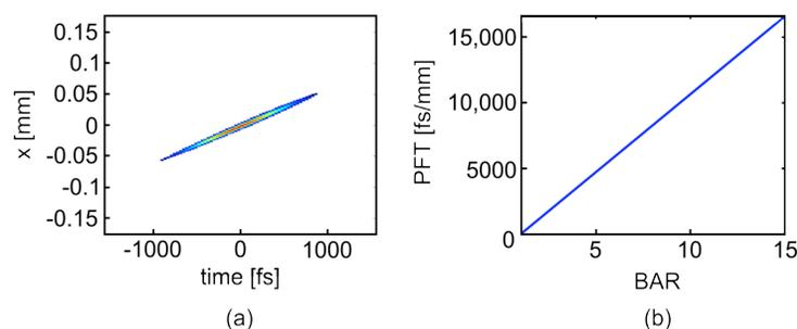
Fig. 2. (a) The simulated spatio-temporal intensity profile of the pulse at the focal plane where  $x$  is the spatial dimension along the direction of spatial chirp. (b) The predicted relationship between the pulse front tilt (PFT) and the beam aspect ratio (BAR) for our system.
